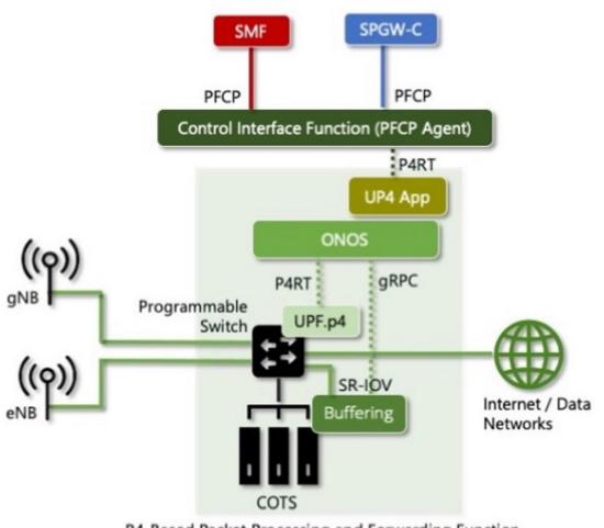
P4-Based Packet Processing and Forwarding Function
