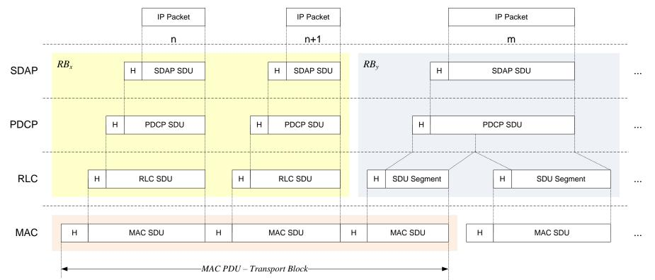
An example of the Layer 2 Data Flow is depicted on Figure 6.6-1, where a transport block is generated by MAC by concatenating two RLC PDUs from  $RB_x$  and one RLC PDU from  $RB_y$ . The two RLC PDUs from  $RB_x$  each corresponds to one IP packet (*n* and *n*+1) while the RLC PDU from  $RB_y$  is a segment of an IP packet (*m*).
